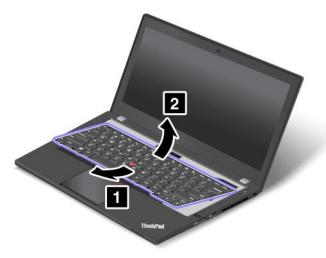
6. Put the keyboard on the palm rest and detach the connectors. Then remove the keyboard.
